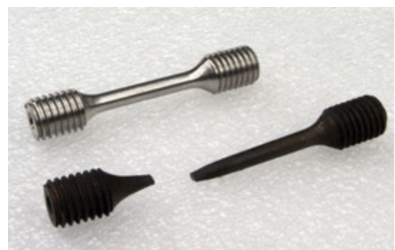
Specimen before and after test
