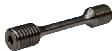
Typical steel specimen for creep test
