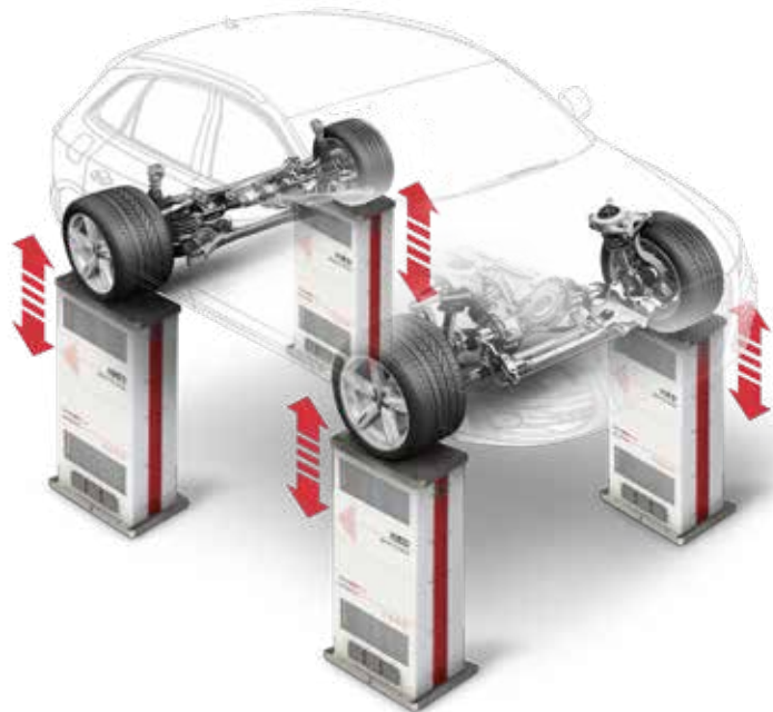
Damper Test System HUD020 with 4 synchronized actuators
