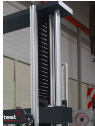
Detail of the screw drivers system and guiding columns in EUROTEST-200 machine
