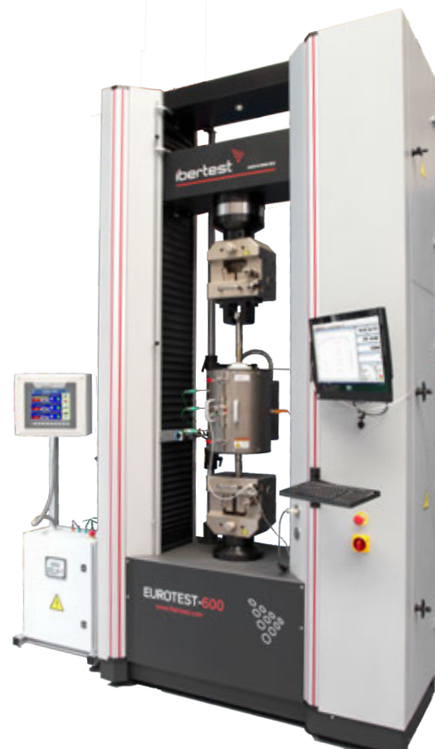
EUROTEST 200 machine with hydraulic side-closing grips and thermal chamber for temperature-controlled tests.
