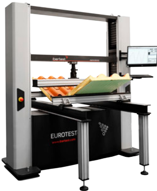
EUROTEST 50 E machine, with extra wide column spacing, removable tensile gripping heads and 3 metre long bending beam.
