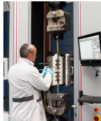
Preparation of high temperature test on EUROTEST-600 machine with high temperature oven.
