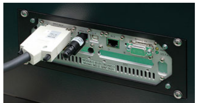
Built-in MD2i module in a Testcom machine
