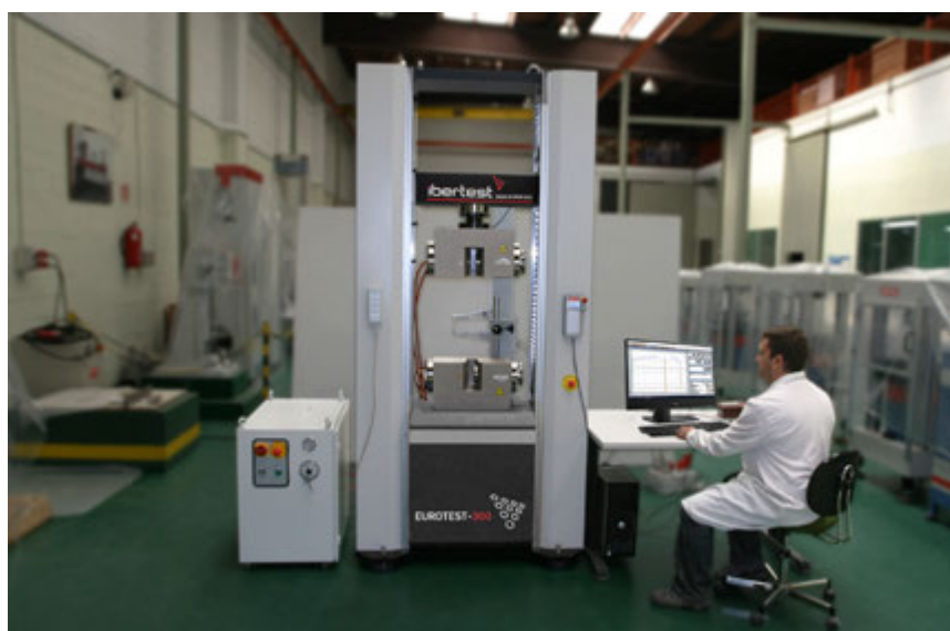
EUROTEST-300 testing machine with lateral close hydraulic grips and long travel extensometer until specimen fracture
