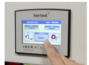
AP-43S electronic module with 4.3" touchscreen display
