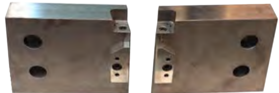
Anvil system with removable radii
