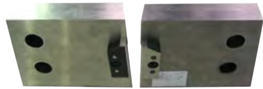
Conventional set of anvils (supplied as standard)
